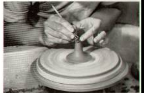
FIGURE 36. The foot is refined to its final shape.
