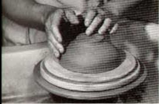
FIGURE 37. When the bowl is leather-hard, it is centered on the wheel.
