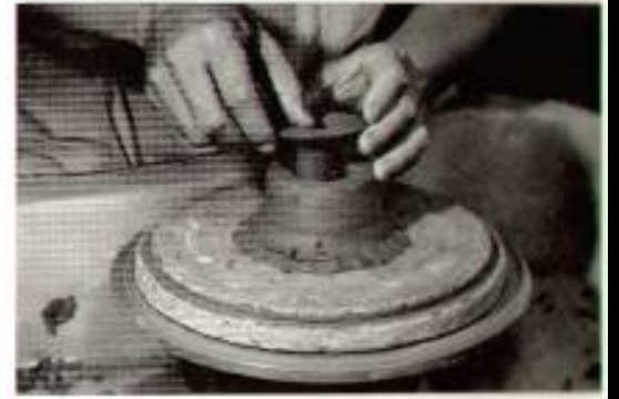
FIGURE 32. When the base of the foot is finished, it is removed.
