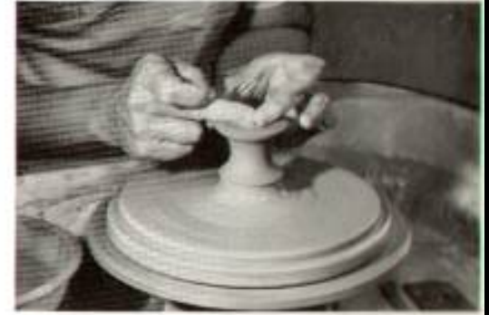
FIGURE 20. The foot is flattened.
