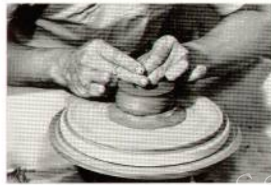
FIGURE 27. As the wheel turns, the support is shaped to run true.
