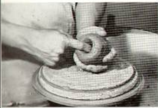
FIGURE 25. A hollow support for the foot is modeled.
