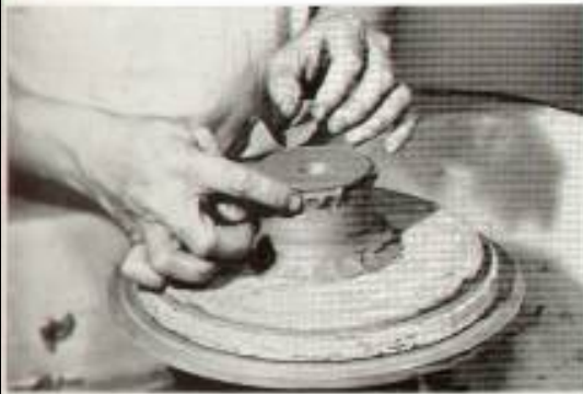
FIGURE 29. The foot is held in position by soft clay.
