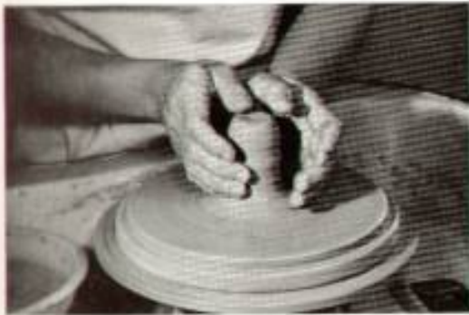
FIGURE 17. This clay is centered and drawn up.
