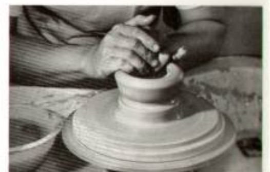
FIGURE 8. The wall is squeezed to broaden and begin to shape the bowl.
