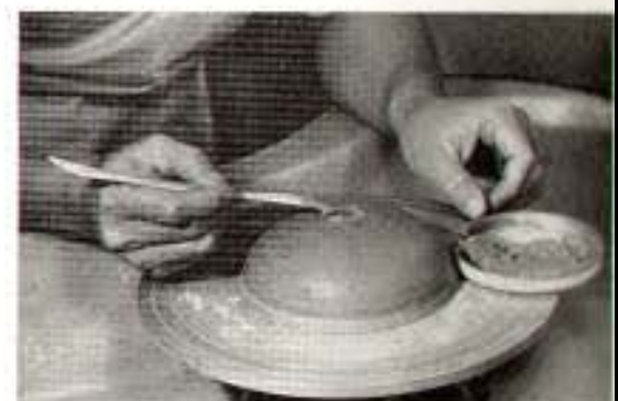
FIGURE 44. Wet clay is applied as a bond.
