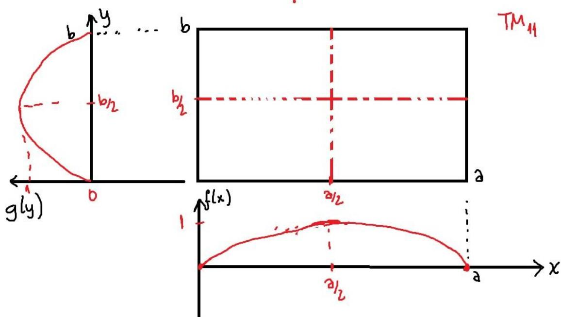
$$E_z(x,y) = A_{nm} \sin\left(\frac{m\pi x}{a}\right) \sin\left(\frac{m\pi y}{b}\right)$$
