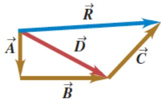
(c) or we could add  $\vec{B}$  and  $\vec{C}$  to get  $\vec{E}$  and then add  $\vec{A}$  to  $\vec{E}$  to get  $\vec{R}$ , ...
