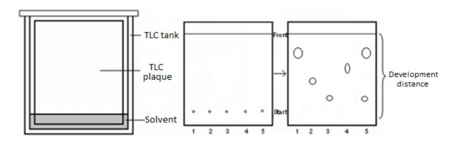
In the example given above, (1-4) standards; (5) sample. It can be said that the sample contains substances (1) and (3).
