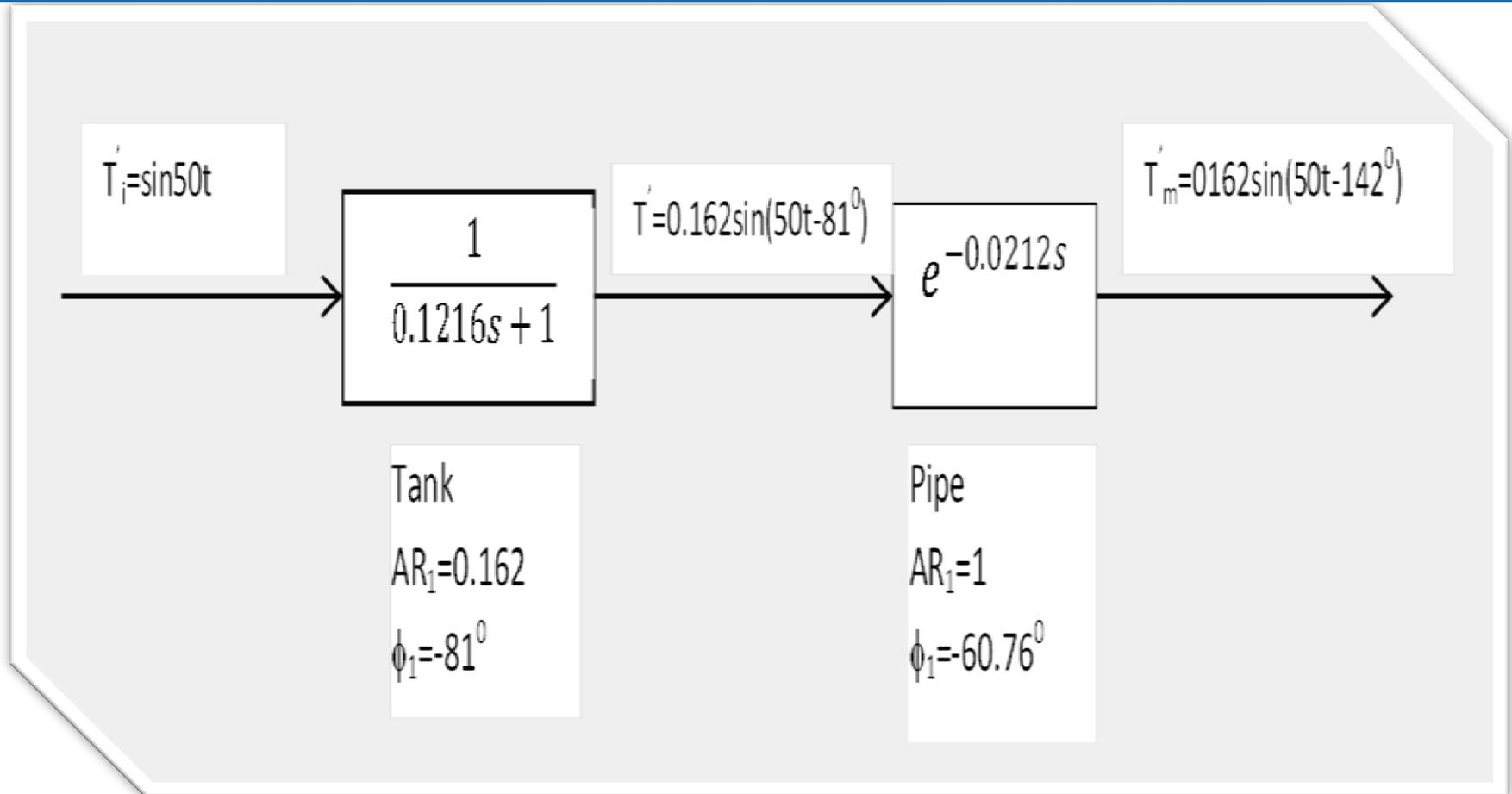
$$\frac{T'(s)}{T_i(s)} * \frac{T_m(s)}{T'(s)} = \frac{T_m(s)}{T_i(s)} = \frac{e^{-0.0212 s}}{0.1216 s + 1}$$
