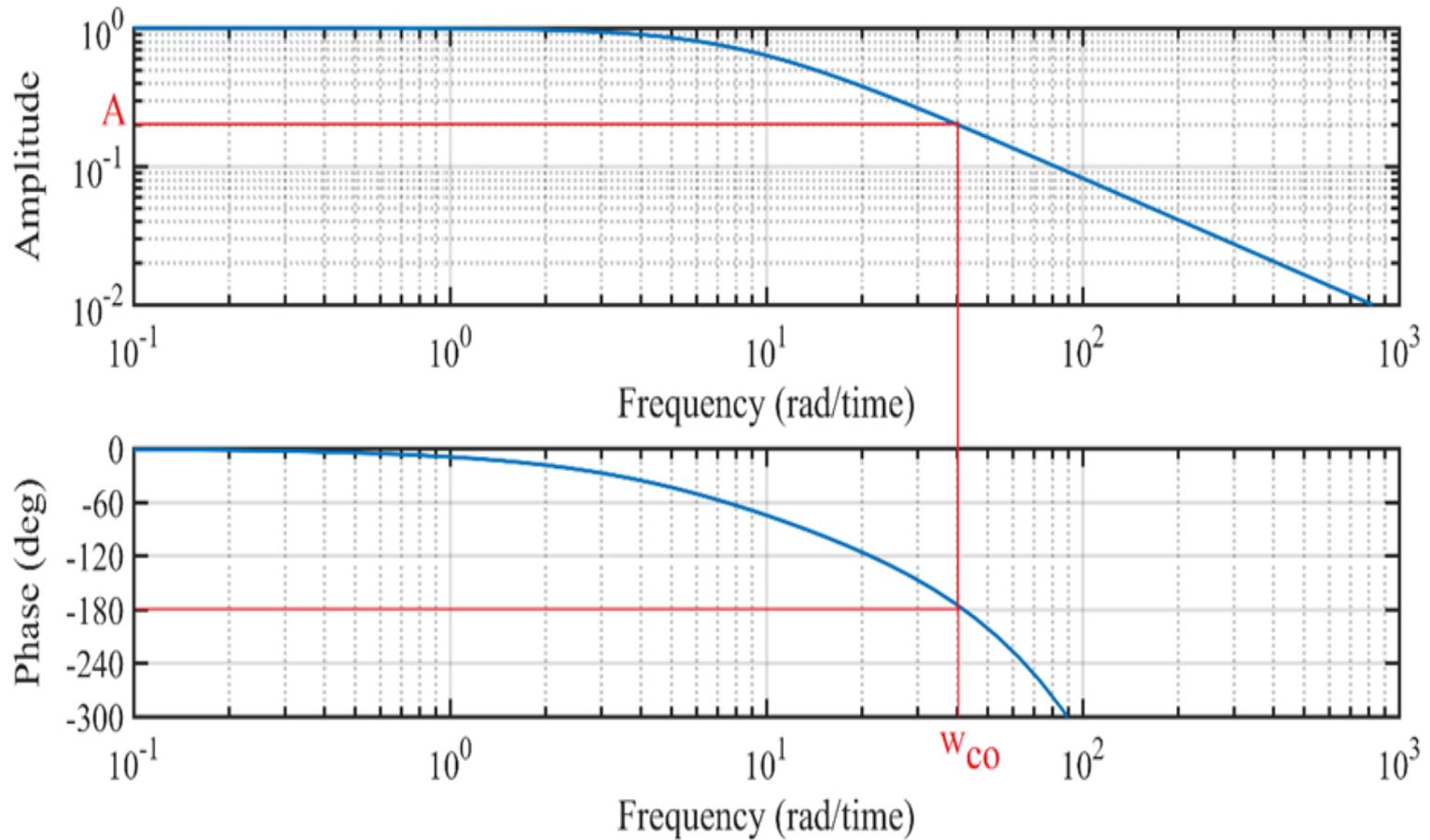
$$\text{At } \phi = -180^\circ \rightarrow w_{co} = 40 \frac{\text{rad}}{\text{min}}$$
