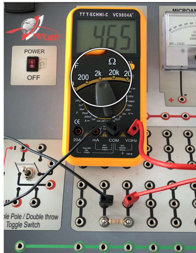
Figure 4. Measuring value of the resistance with the Avometer.
