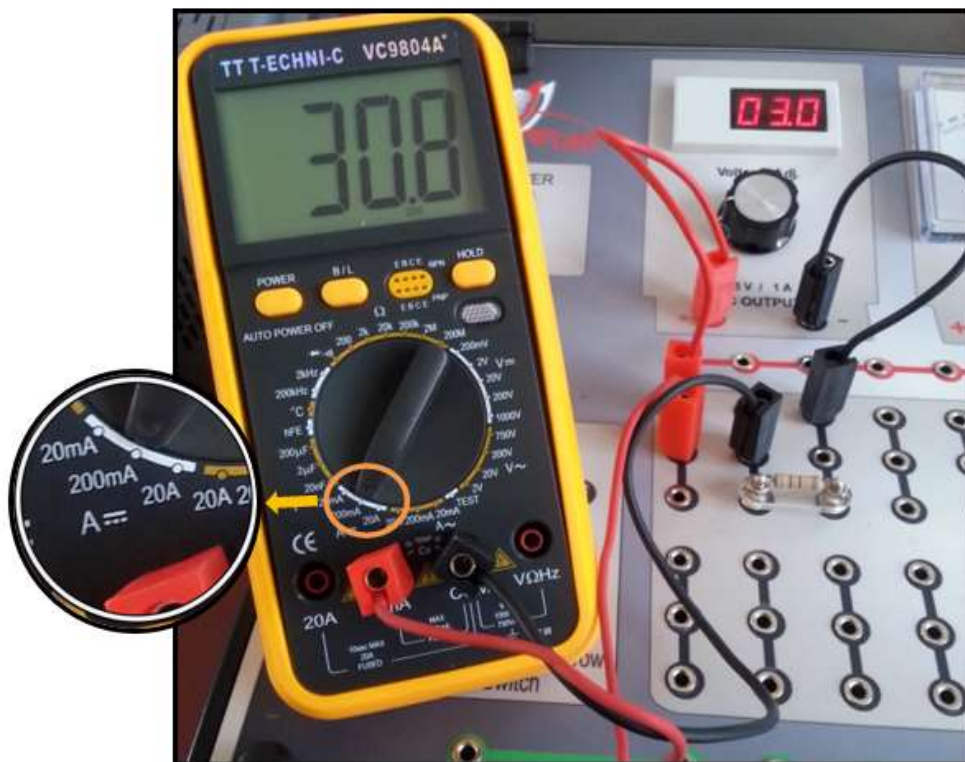
Figure 3. Measuring the current value of the resistance with the avometer.
