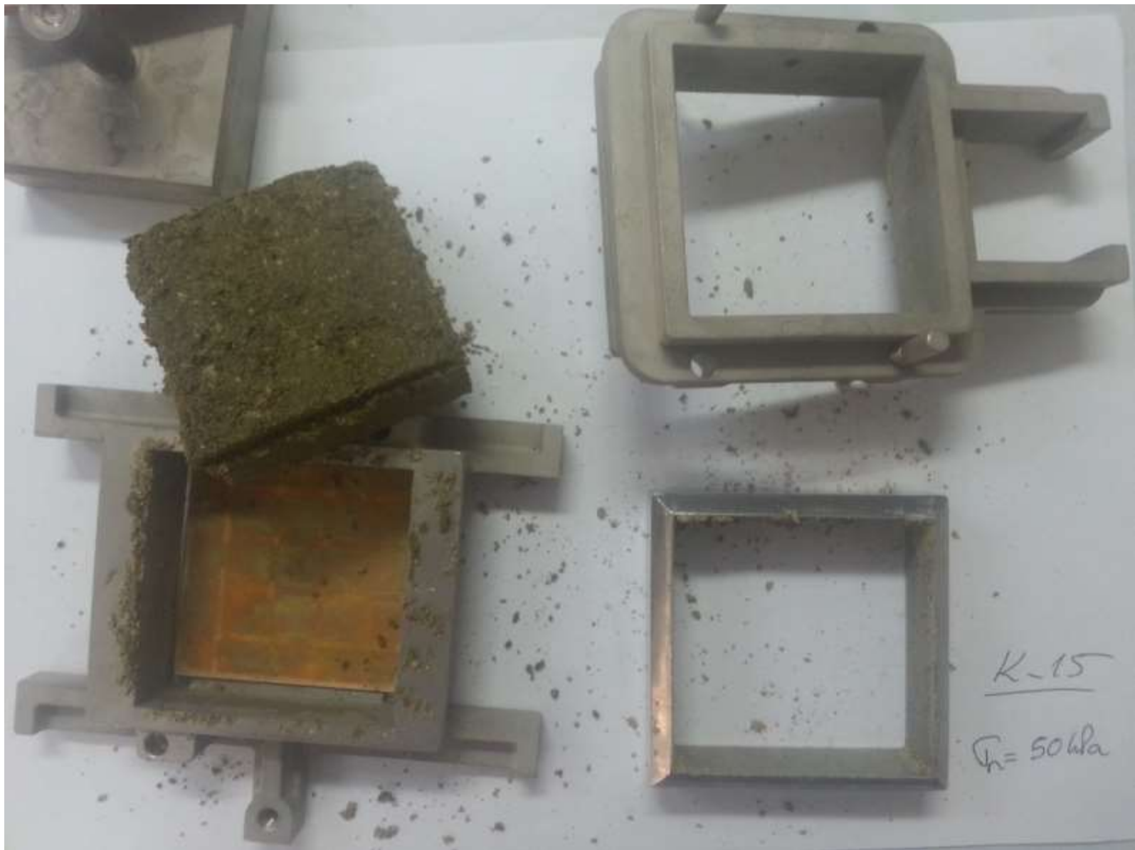
Soil sample after shearing stress is applied
