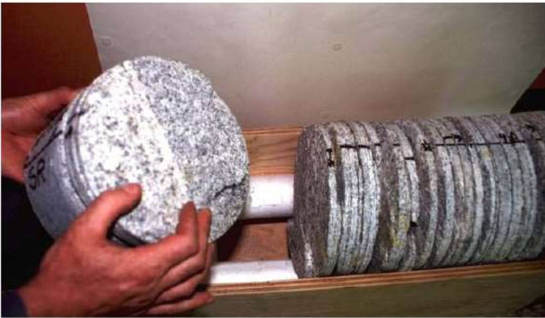
Figure 1.7: Disking of a 150 mm core of granite as a result of high in situ stresses.
