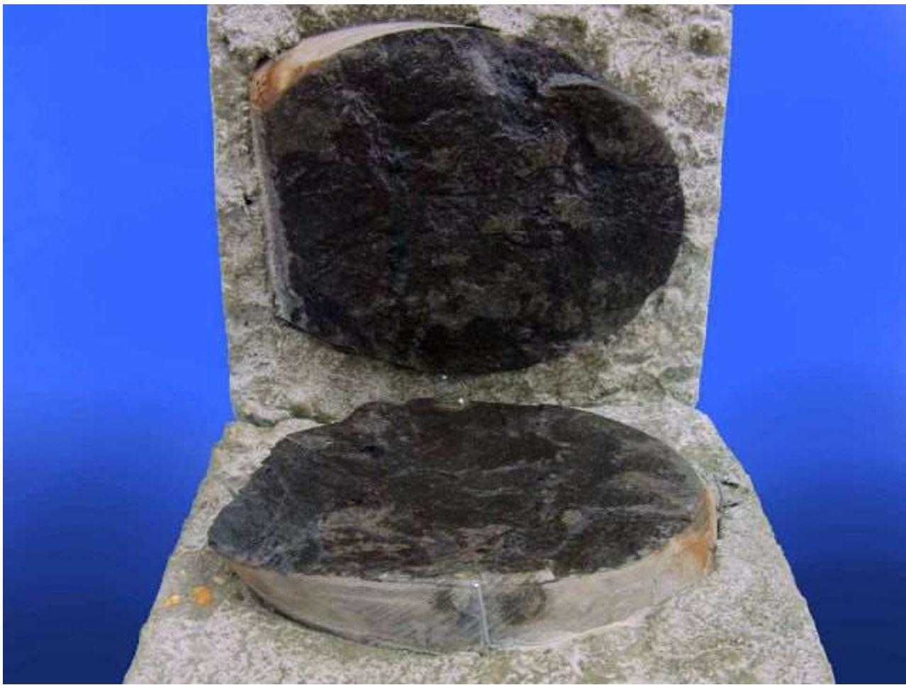
Interface failure on the geopolymerside
