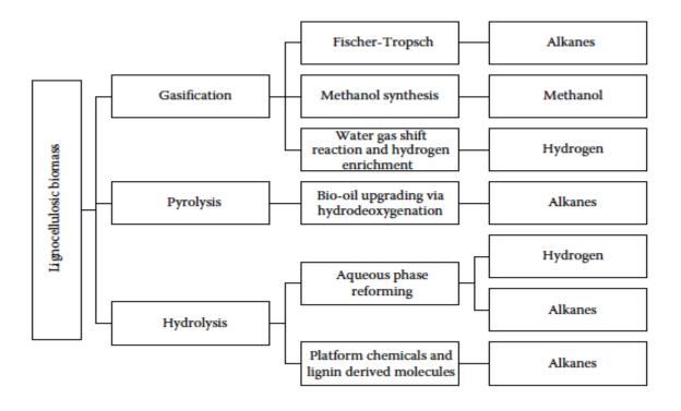
The three portions are processed together through strategies like gasification and pyrolysis, offering simplicity of operation, and lower operating costs. The alternative approach is to separate the three fractions of lignocellulose from each other by adopting various pretreatment strategies and process them separately.
