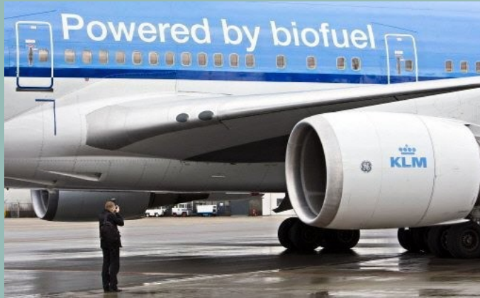
A Boeing 747, one of four engines powered by a 50-percent biokerosene mix.
