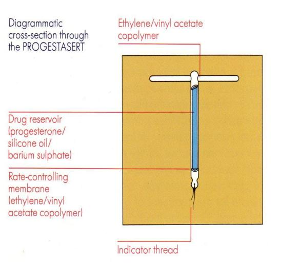
However, since the device delivers progesterone to its target ulletlocally at a rate of approximately 65 pg/day, the system lasts for over 1 year. Marketed by ALZA under the trade name Progestasert ®, the system showed comparable pregnancy and expulsion rates to conventional IUDs, often with less menstrual bleeding.
