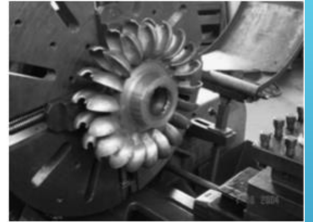
FIGURE 2.25 A 100-kW Pelton turbine in a workshop, Nepal.
