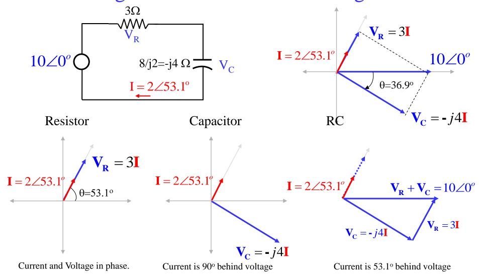
The phasor diagram representation shows the phase vector of three voltages and one current. Note that the sum of  $V_R$  and  $V_C$  constitutes the source voltage and vector.  $V_C$  is 90° behind I;  $V_R$  is in the current direction (in phase).
