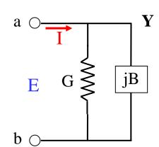
**Example-5.4:** Angular frequency of the driving source is 10 rad/s, find the input impedance of the following circuit.
