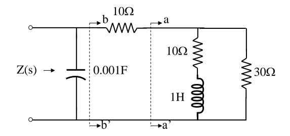
To the right of line aa', the  $30\Omega$  resistor is parallel to the  $10\Omega$  resistor and the series arrangement of the 1H coil. Impedance of series:
