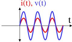
Voltage and current are in the same phase - where one is maximum and the other is maximum. (Plotted for R>1)
