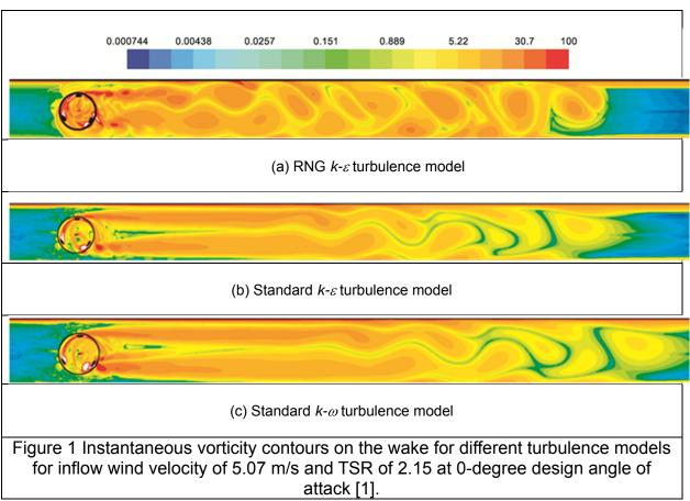
The less elongated separated shear layer in case of the RNG k-ε model leads to stronger and more discernible vortex patterns in the wake compared to those for the other two standard turbulence model cases, which reproduce more elongated separated shear layers rolling into very weak and less discernible vortex patters as seen in Figs. 1(b) - (c) [1].
