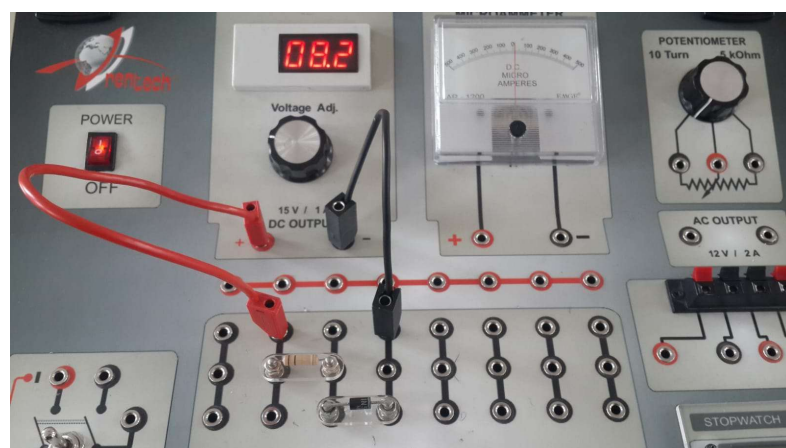
Figure 6.6 Semiconductor diode experimental setup
