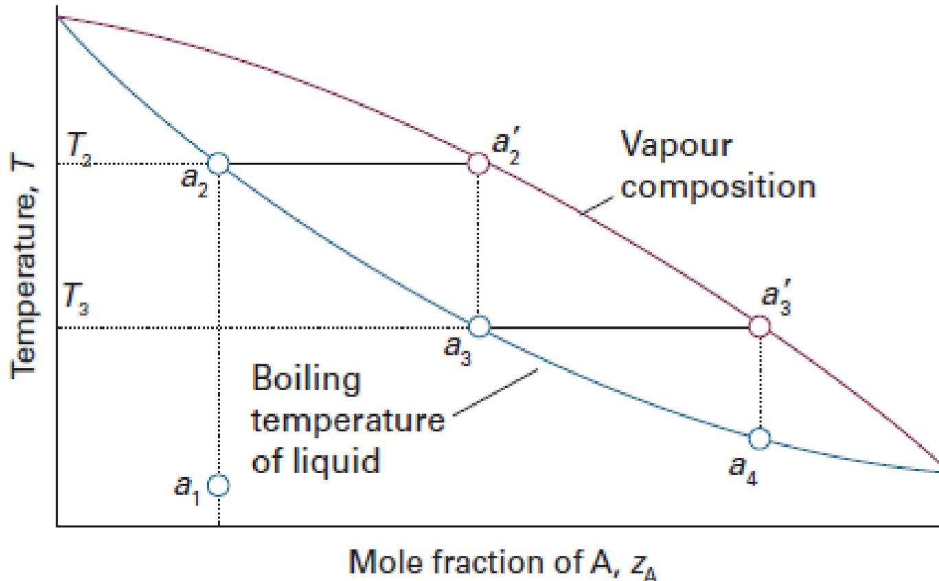
**In a simple distillation**, the vapour is withdrawn and condensed. This technique is used to **separate a volatile liquid from a non-volatile solute or solid**.
