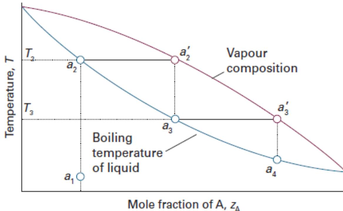
Successive boilings and condensations of a liquid originally of composition  $a_1$  lead to a condensate that is pure A. The separation technique is called **fractional distillation**.
