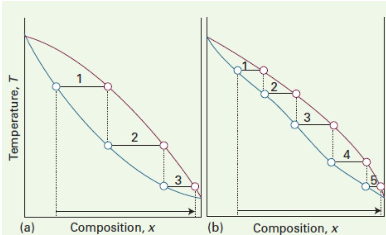
In figure a, the fractionating column must correspond to **three theoretical plates**.
