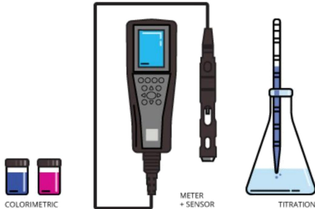
Dissolved oxygen can be measured by colorimetry, a sensor and meter or by titration.
