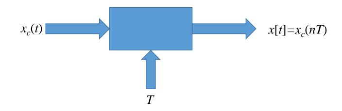
Ideal Continuous-Time to Discrete-Time (C/D) Converter
