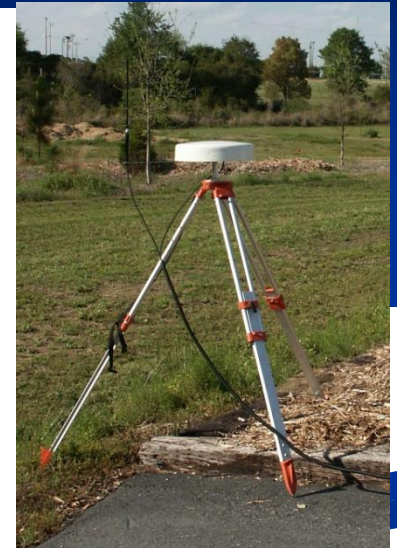
DGPS Base Station with Radio (on RTK systems only)
