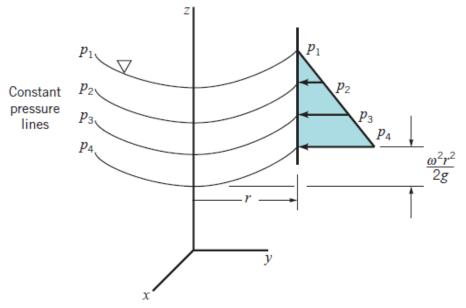
Figure 3.36. Pressure distribution in a rotating liquid.
