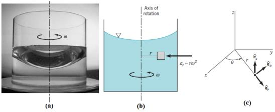
Figure 3.35. Rigid-body rotation of a liquid in a tank.
