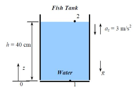
(a) Tank stationary: We have az = 0, and thus the gage pressure at the tank bottom is
