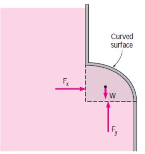
Figure 3.31. When a curved surface is above the liquid, the weight of the liquid and the vertical component of the hydrostatic force act in the opposite directions
