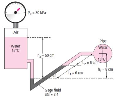
**Solution:** The specific gravity of gage fluid is given to be 2.4. We take the standard density of water to be  $\rho w = 1000 \text{ kg/m}^3$ .
