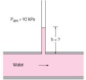
**Solution:** A glass tube open to the atmosphere is attached to a water pipe, and the pressure at the bottom of the tube is measured. It is to be determined how high the water will rise in the tube. The pressure at the bottom of the tube can be expressed as
