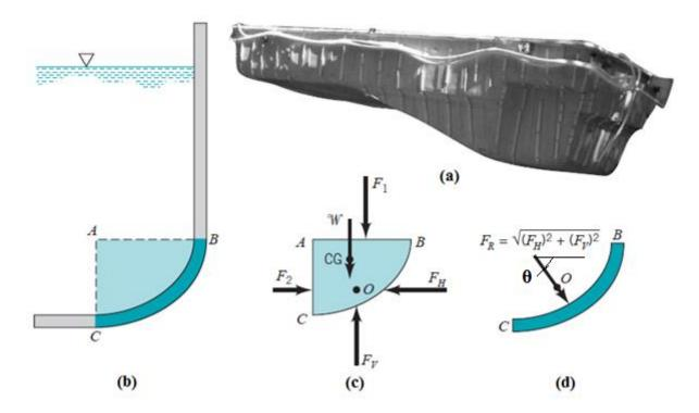
Figure 3.30. Hydrostatic force on a curved surface.
