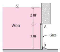
**Solution:** The average pressure on a surface is the pressure at the centroid (midpoint) of the surface, and multiplying it by the plate area gives the resultant hydrostatic force on the gate,
