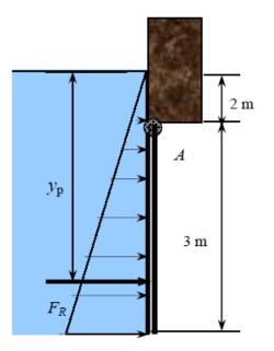
b) The hydrostatic force exerted on the gate for a total water height of 2 m. The average pressure on a surface is the pressure at the centroid (midpoint) of the surface, and multiplying it by the wetted plate area gives the resultant hydrostatic force on the gate,
