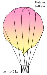
a) The density of air is given to be  $\rho = 1.16 \text{ kg/m}^3$ . The density of helium gas is 1/7th of this. The buoyancy force acting on the balloon is
