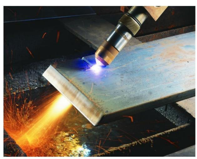
Figure 2. A plasma torch can be used to cut metal. (credit: "Hypertherm"/Wikimedia Commons)
