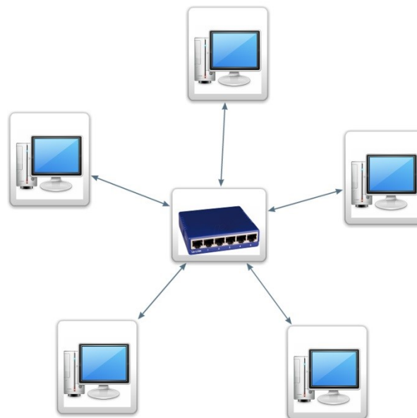
Figure 6: Graph Representation of Star Topology
