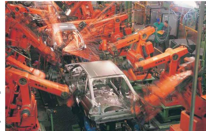
Robotic welding along an automobile assembly line. Increased automation has reduced labor requirements in secondary industrial
