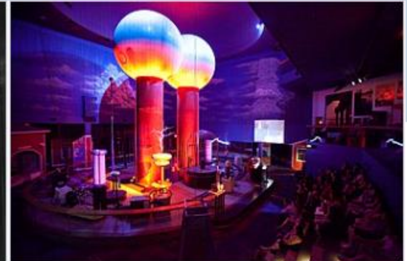
An educational program at the Theater of Electricity, Boston Museum of Science demonstrates the world's largest air-insulated Van de Graaff generator, built by Van de Graaff in the 1930s.
