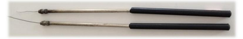
The wire assembly can be ring-curled, straight or hooked, depending on the purpose of use.
