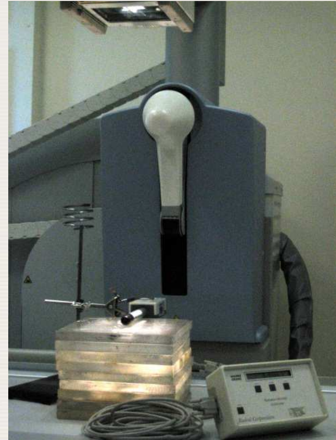
Measurement of entrance surface air kerma using PMMA slab
