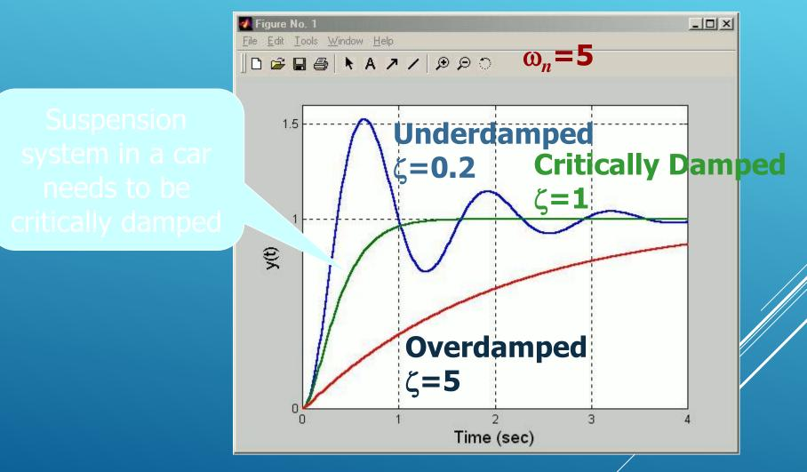
Transient Response Analysis Second Order Systems, R(s)=1/s Underdamped Case (0<ζ<1)
