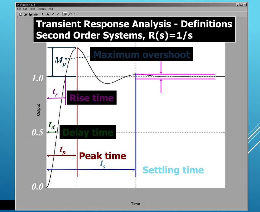
Delay Time  $(t_d)$ : The time required to reach the half of the final value. Note that delay time is the time till first reach is observed.
