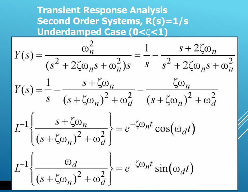
Transient Response Analysis Second Order Systems, R(s)=1/s Underdamped Case (0<ζ<1)
