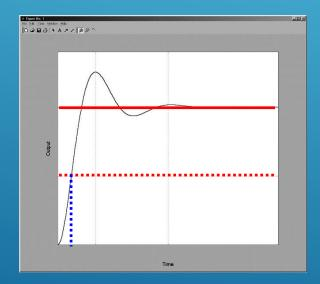
Rise Time ( $t_r$ ): The time required to rise from 10% to 90% or 5% to 95% or 0% to 100% of the final value.
