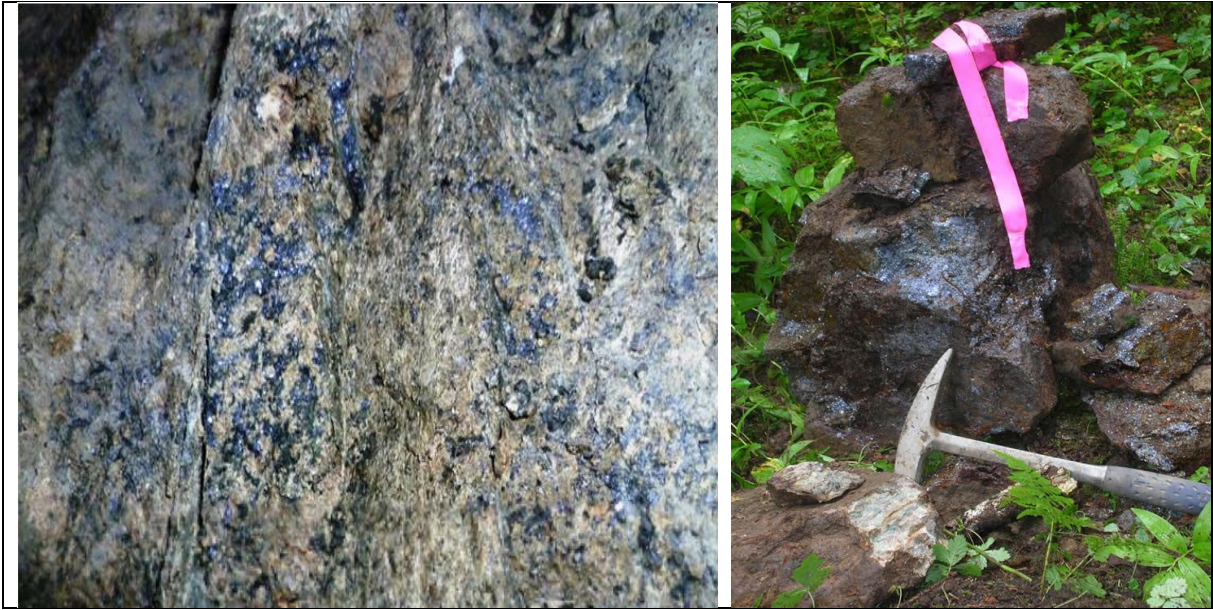
Molybdenite (MoS 2 ) mineralization in garnetiferous skarn High grade molybdenite in skarn. Up to 12% Molybdenum
