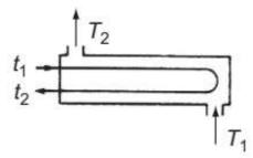
• Temperature correction factor; one shell pass; two or more even tube passes
