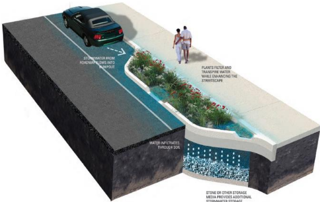
Mid-block Stormwater Bump-out
