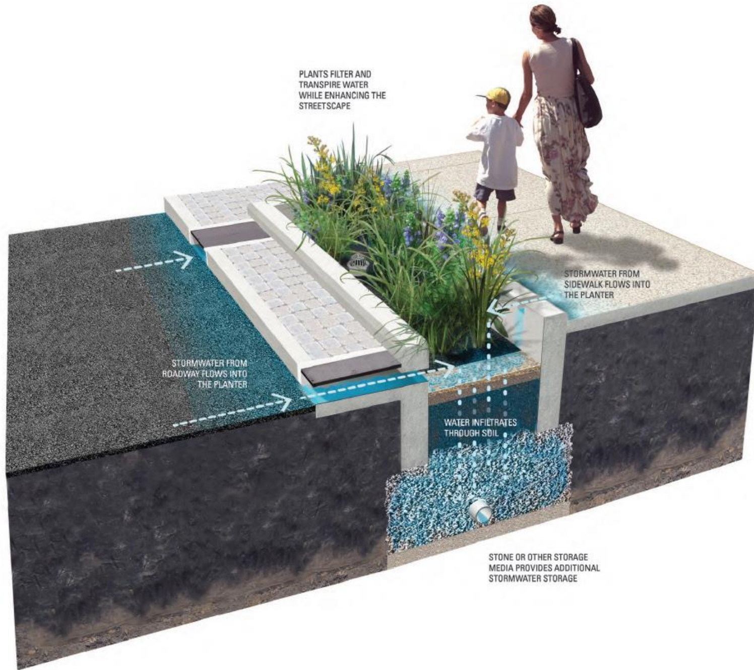
Figure 2.1: Three-Dimensional View of a Stormwater Planter
