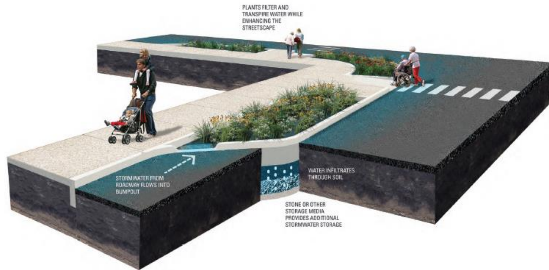
Corner Stormwater Bump-out
