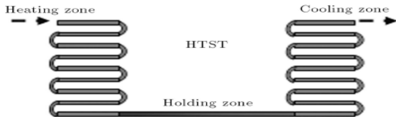
Figure 1. Schematic diagrams of HTST and UHT processes.
