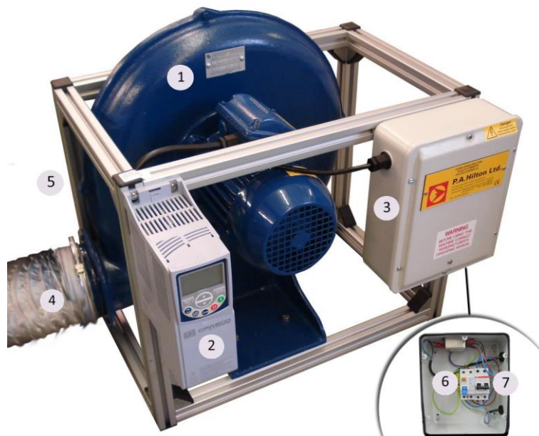
General experimental setup of Airflow System: 1. Fan; 2. Fan Speed Control; 3. RCCB & MCB Box; 4. Fan Outlet; 5. Fan Inlet; 6. RCCB; 7. MCB
