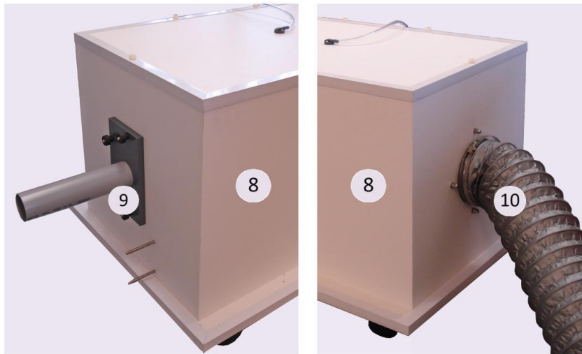
General experimental setup of Plenum Chamber: 8. Plenum Chamber; 9. Plenum Discharge; 10. Plenum Inlet
