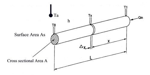
A pin of length L diameter D and cross-sectional area A (Perimeter P) and thermal conductivity kis heated at one end. It has a total surface area As and is in an ambient at temperature Ta.
