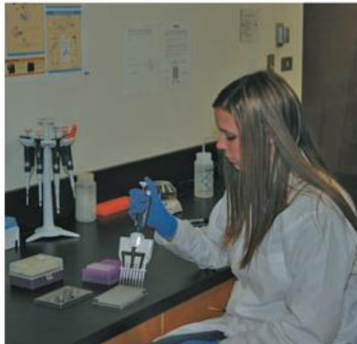
(a) A technician uses a micropipette to add samples to a microplate for an ELISA.
