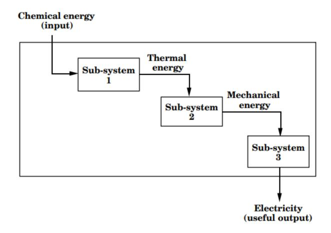
One of the most important energy conversion systems in our modern society is the electric power plant. The chemical energy is first converted to thermal energy in the boiler; thermal energy is then converted to mechanical energy in the turbine; finally, mechanical energy is converted to electricity in the generator. System efficiency is, therefore,
