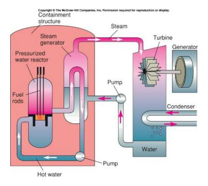
As with nuclear bombs, the primary fuel is uranium-235. Uranium ore is enriched and formed into fuel pellets. The fuel pellets are stacked into long, cylindrical fuel rods. Control rods, made of a neutron-absorbing material, are placed amongst the fuel rods. They can be removed and inserted to adjust the rate of the chain reaction. Withdraw control rods, reaction increases:
