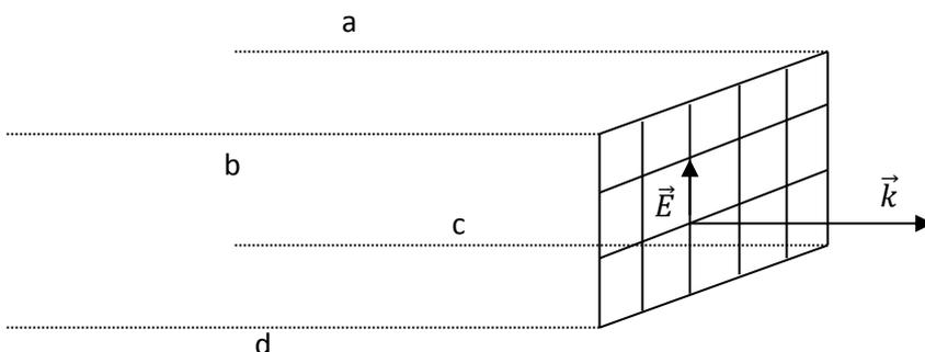
A uniform plane wave is a particular solution of Maxwell's equation assuming electric field (and magnetic field) has same magnitude and phase in infinite planes perpendicular to the direction of propagation. It may be noted that in the strict sense a uniform plane wave doesn't exist in practice as creation of such waves are possible with sources of infinite extent. However, at large distances from the source, the wavefront or the surface of the constant phase becomes almost spherical and a small
