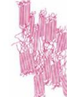
4. Separation of crystalline block segments during the third stage
