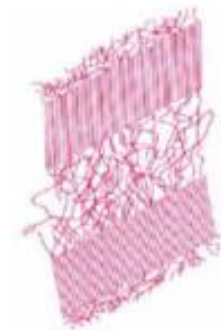
3. Tilting of lamellar chain folds during the second stage
