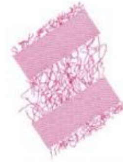
2. Elongation of amorphous tie chains during the first stage of deformation
