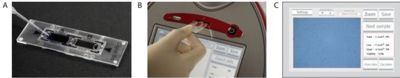
Figure 1—Countess™ Automated Cell Counter. The Countess™ Automated Cell Counter eliminates the tedium and subjectivity of manual cell counting. Automated counting frees up your time, reduces eye strain, and minimizes subjective judgments that can lead to error. It takes 3 simple steps: (A) Mix 10 \mu L of sample with 10 \mu L of trypan blue, and pipet into Countess™ chamber slide. (B) Insert slide into the instrument. (C) Press the “Count cells” button, and results are displayed in 30 seconds.
