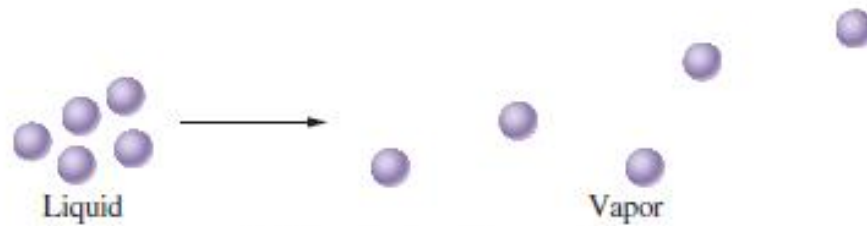
(b) Vaporization: S_{\text{vapor}} > S_{\text{liquid}}
