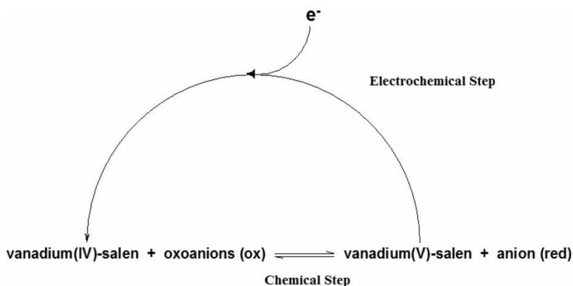
**Scheme 1.** Response of the Vanadium(IV)-Salen modified electrode for the catalytic reduction of various oxoanions.
