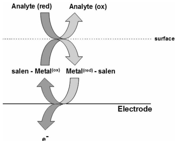
**Figure 4.** Schematic representation of electrocatalysis at a metal-salen modified electrode. ox = oxidized species and red = reduced species.
