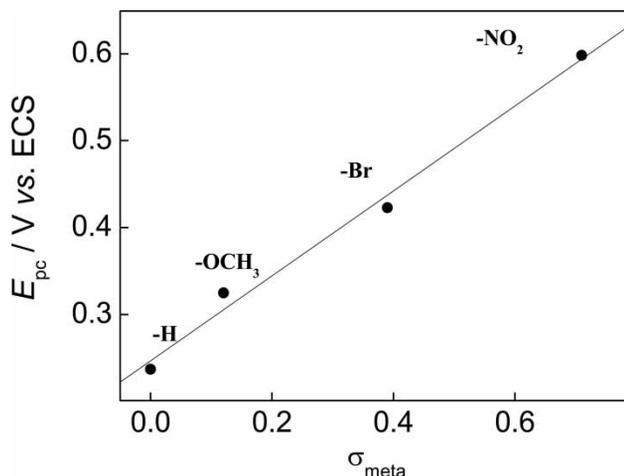
**Figure 5.** Cathodic peak potential of the carbon paste electrode modified with VO(X-Salen) vs. Hammett constant (Teixeira et al. 2005).
