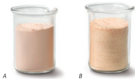
The cell culture medium produced by Merck Millipore (A) appears as a homogenous powder, whereas the cell culture media of other suppliers (e.g., B) show crystals and inhomogeneous blending.
