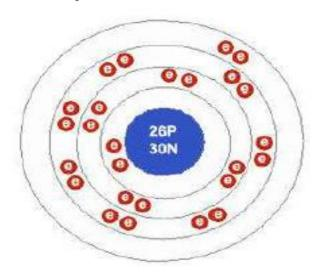
This iron atom (26 protons, 26 electrons) has two electrons in its outer shell, which can move from one iron atom to the next in a metal.
