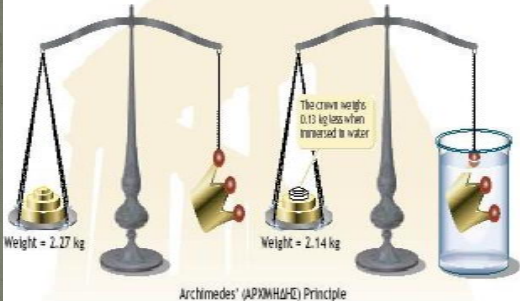
FIGURE 28.8 • Archimedes' principle of buoyant force to determine the volume and, subsequently, specific gravity of the king's crown.
